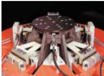
Figure 1. The photo shows the lightweight armature and suspension arrangement on the V875-240.
