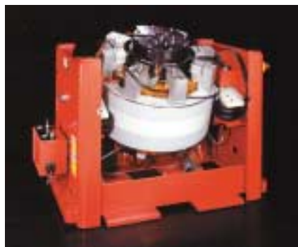
Figure 4. The photo shows the armature and suspension arrangement on the V9 High Force Shaker.
